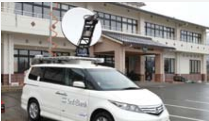
Mobile base station vehicle
