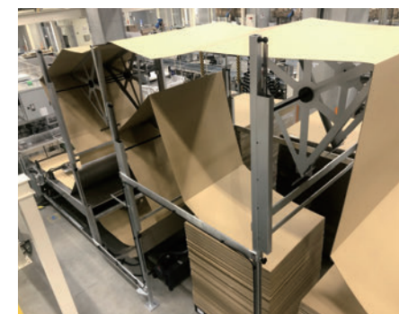
Packaging machine that automatically generates boxes with three adjustable sides
