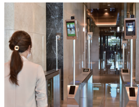
Facial-recognition entry-exit system with a temperature-sensing function
